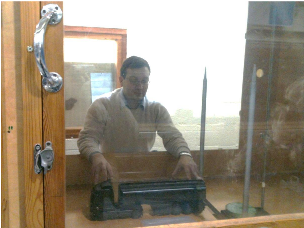
Figure 2 : A researcher puts a lorry model inside a wind tunnel for tests.
