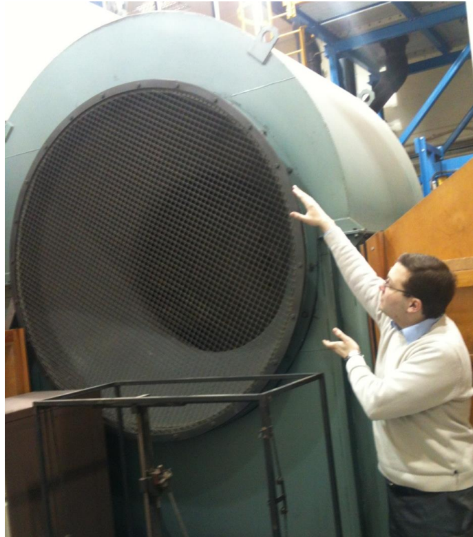
Figure 4 : The Inlet duct of the blowing fan for the wind tunnel its reasonably large.
