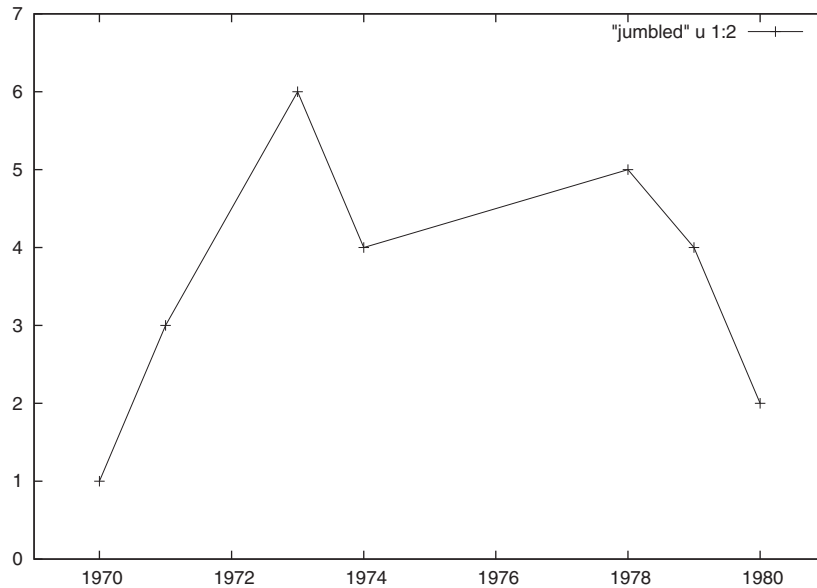
Figure 3.2 Using smooth unique lets us sort x values on the fly: plot "jumbled" u 1:2 smooth unique with linespoints
